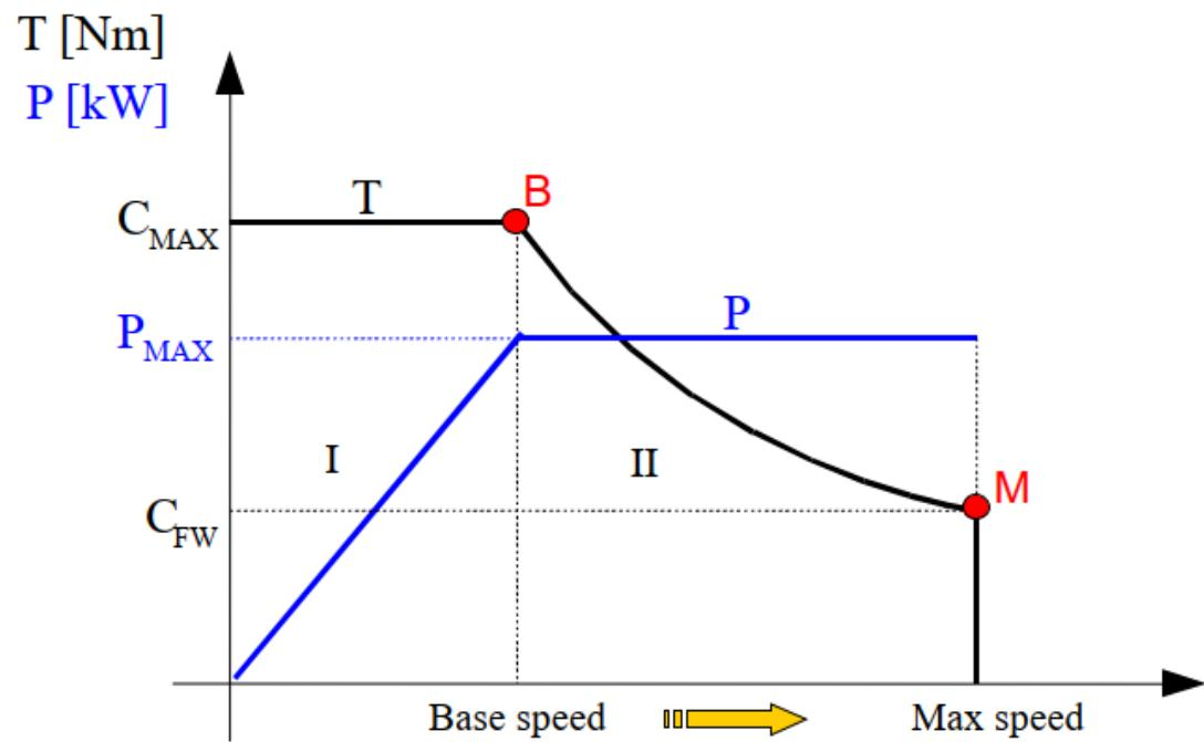
**At low speeds:** The torque is ideally constant up to the base speed. The dissipated energy is dominated by the copper losses, while the core losses in the iron are relatively low.
